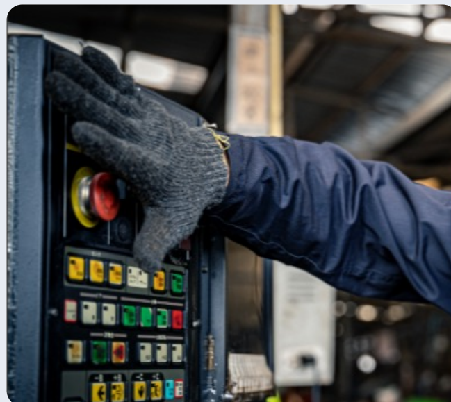
Figure 8: E-stops must be initiated by a single human action
