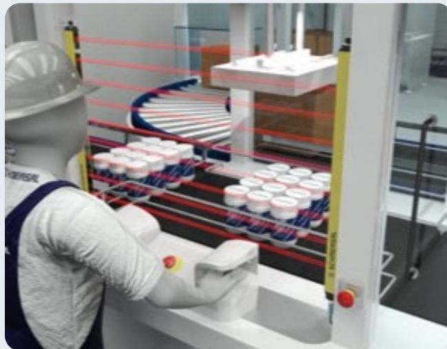
Figure 8: E-stops must be initiated by a single human action
